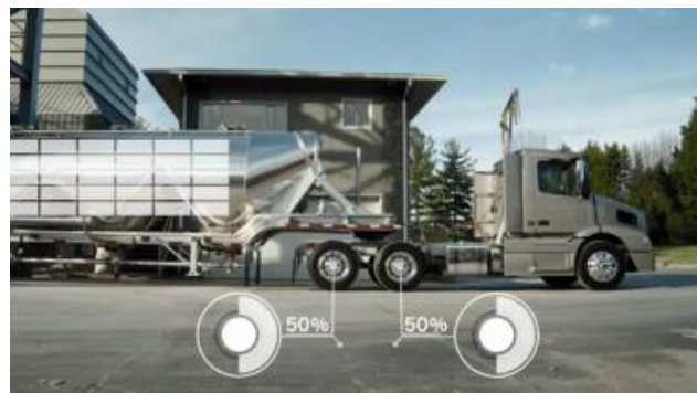
Figure 1: Distribution of Weight to Axles in a 6x4 Configuration
