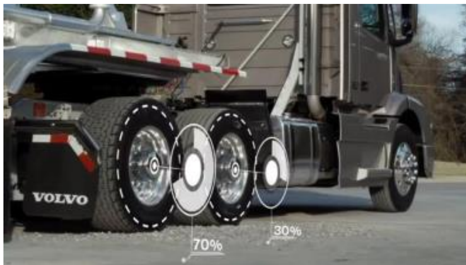
Figure 2: Distribution of Weight to Axles in a 6x2 Configuration
